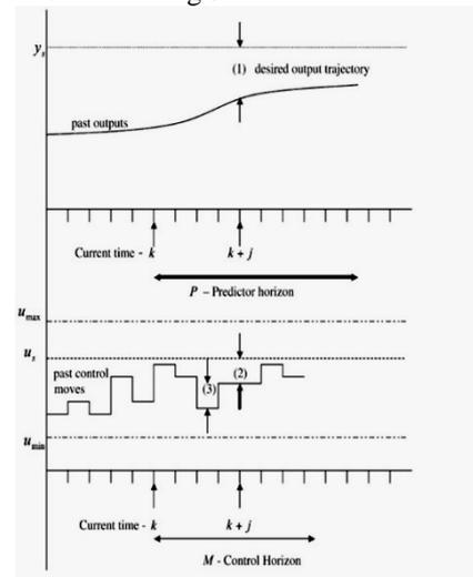
Fig 3 Schematic representation of the MPC control algorithm
