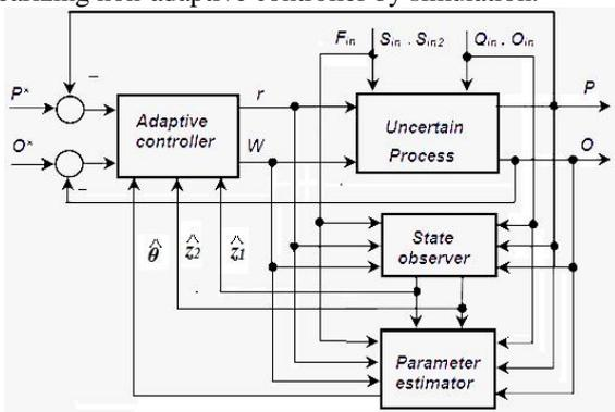
Fig 8 Block diagram of the designed adaptive system
