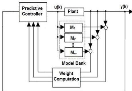
Fig 4 Multiple-model (including locally linear neuro-fuzzy models) structure
