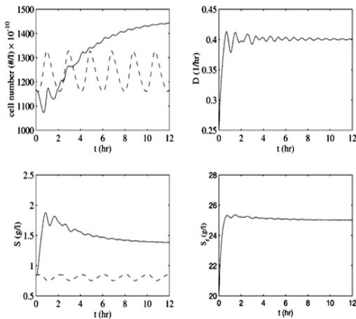
Fig 2 Oscillation attenuation: reduced-order output vector without disturbance model (-) and open loop response (- -)
