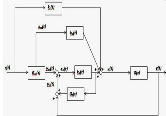
Fig 9 SAC system with parallel feed forward controller
