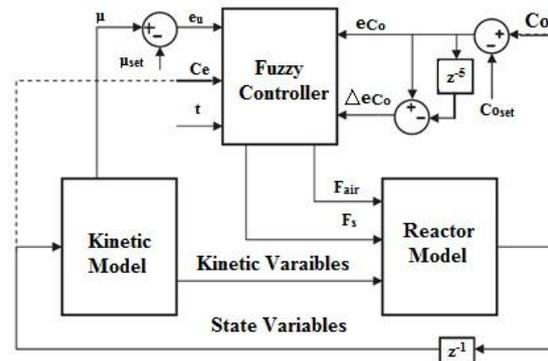
Fig 11 Block diagram of the control structure
