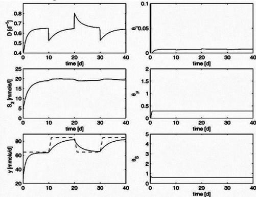
Fig 7 Anaerobic digester Performance of the extremum seeking control
