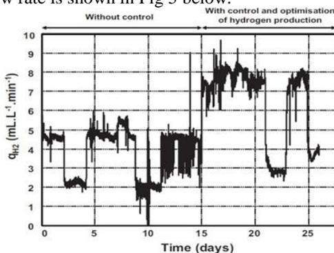
Fig 5 Hydrogen gas flow rate with and without control
