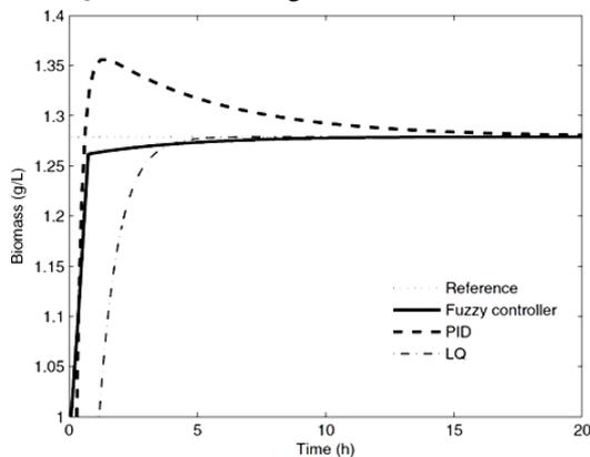
Fig 13 Comparison of the biomass fuzzy servo controller with PID and LQ controllers
