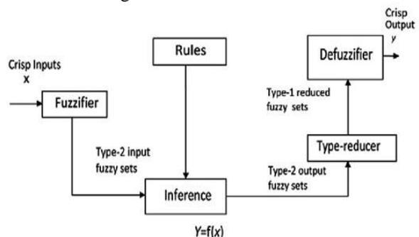
Fig 12 Type-2 Fuzzy logic controller
