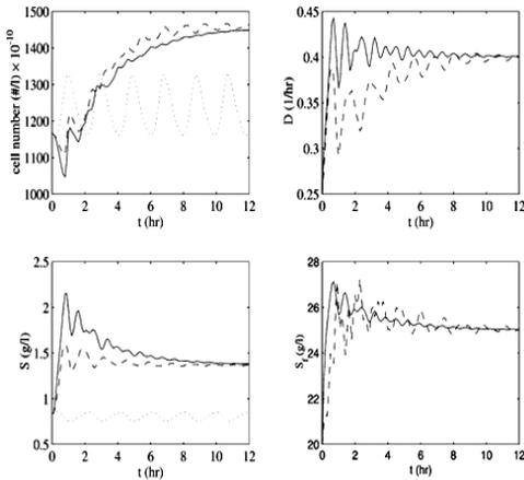
Fig 1 Oscillation attenuation: full-order output vector with (- -) and without (-) disturbance model and open loop response (.....)
